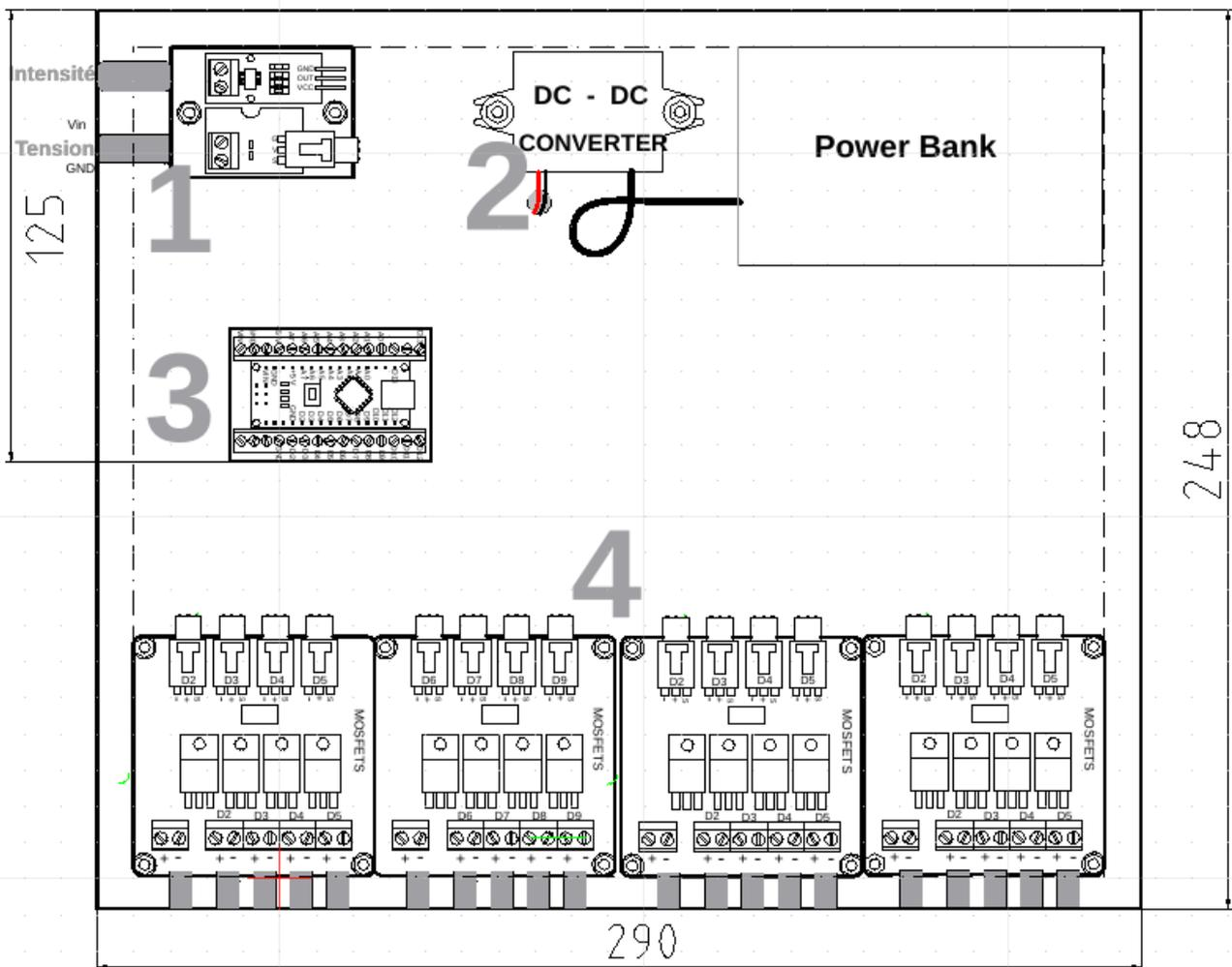
Make sure that there are sufficiently comfortable passageways, so that the cables do not have to be twisted.
